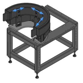
b. Loosen the four (4) screws on each of the three stands.
