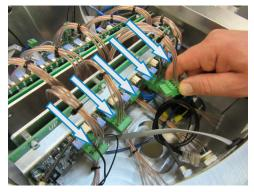
6. Remove the fourteen (14) screws that secure the board to the bus bar.
