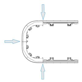
Adjust the vertical, horizontal, and side-to-side positions until the upper v-rails align with the straight sections, and the curved section is centered between the straight sections.
