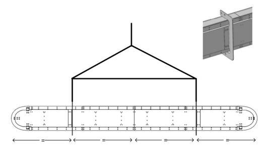
Remove from shipping box using the upper two holes on each lifting bracket. Use of a spreader bar is required.
