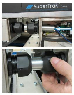
4. Feed the required wiring through the metal conduit and connect as required, then close the sections' electrical doors.
