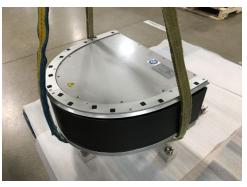
3. When the 180 deg. section is in the required position, remove the lifting straps.
