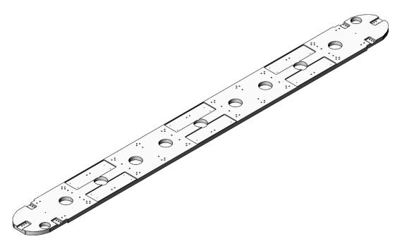
2. Position the base plate across two (2) or more metal saw horses, with the slotted cut-outs facing up.
