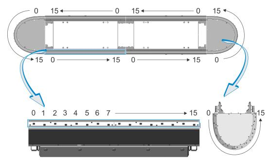
Each 180 deg. section (800 mm) has four (4) encoder assemblies: a left encoder assembly, two (2) center encoder assemblies, and a right encoder assembly. The functionality is the same as described above except that the encoders are numbered 0 to 7 from left to right, as pictured at right.
