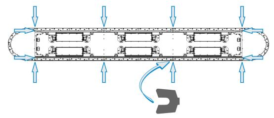
Install the wedge adjust for the 180 deg. sections.
