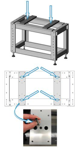
e. Secure the cross-brace in position with four (4) screws.
