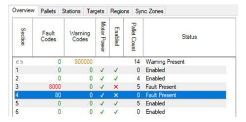
2. Gateway network error as seen from the Fault/Warning Message List of the Overview tab of the right panel in the System Dashboard view.
