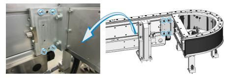
c. Turn the wedge adjustment knob, as required, to adjust the upper v-rail in or out.
