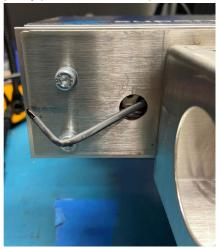
5. Replace the thermistor at the end of the wire.
