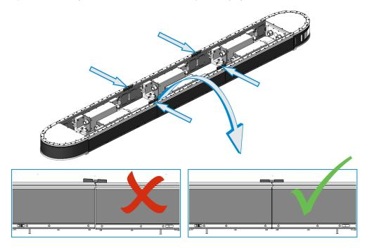
11. Install a wedge adjust between each of the straight sections.
