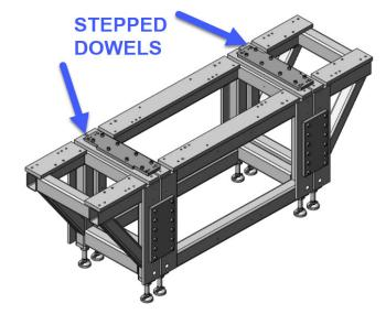
5. Install four (4) screws in the top connection plate to secure it in position.
