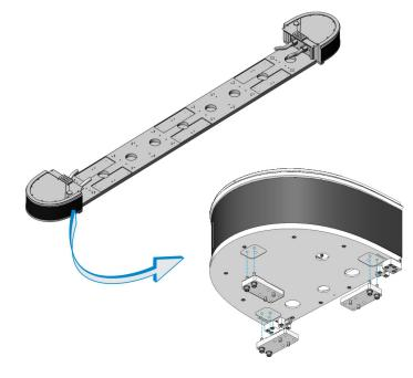
b. Align the 180 deg. section with the base plate, and then secure with twelve (12) screws.
