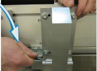
b. Loosen the four (4) wedge screws.
