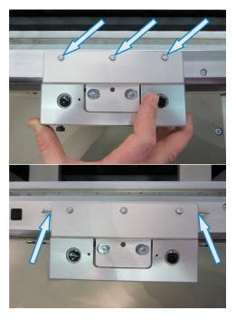
5. Install the shuttle below the removable locate.
