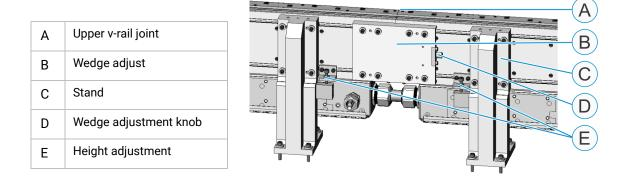
1. Choose a track section on which to base alignment for other sections as a starting point, then tighten all eight wedge screws on that section.
