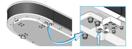
15. Tighten the four (4) screws in each straight section stand base.
