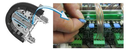
5. Install a new 15A fuse straight into the fuse slot.
