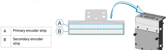
Align a shuttle encoder strip assembly if the encoder strip is removed during maintenance, or if the shuttle position faults regularly occur on the curved section.
