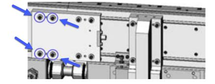
2. Now tighten the four wedge screws on the next section over.
