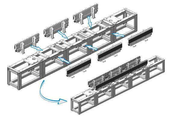
4. Position all straight sections on the frame, with the electrical box facing out.
