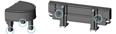
4. Install two (2) dowels through the outer holes of top connection plate, to position the top connection plate on the frame.
