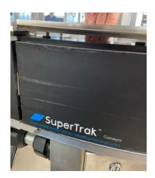
9. Clean the top of the section with a soft cloth to remove any debris.
