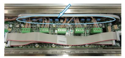
6. Install a new 15A fuse straight into the fuse slot.
