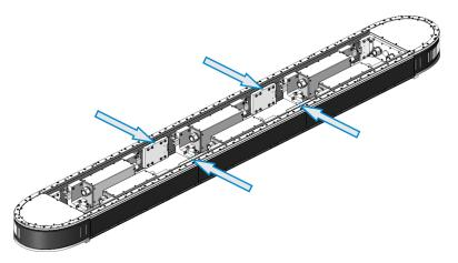
13. Align the upper v-rails by adjusting the wedge or adjusting the screws on the inside of the 180 deg. section.
