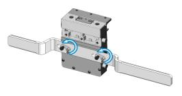
4. Lift the shuttle using the handles of the shuttle removal tool.
