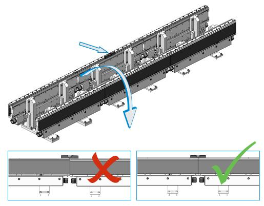
11. Install a wedge adjust between the straight sections.
