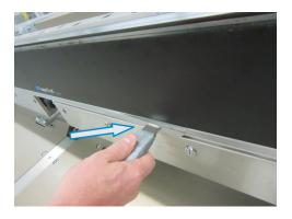
3. Holding onto the magnet, pull the wear strip straight out of the channel.
