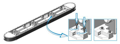
16. Add wear strip locators to straight sections with the tabs directed towards the center of the each section.
