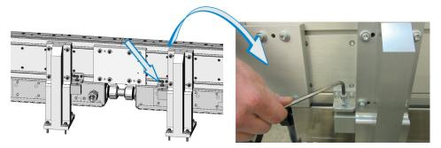
d. Tighten the four (4) stand screws and four (4) wedge screws that were loosened in step a and b.
