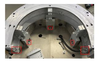
6. Loosen the adjacent straight sections' V-rails. Do not remove them completely, but loosening them will make it easier to install the new V-rails on the 180 deg. (800) section.
