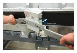
6. Hold the shuttle level. With the anti-tip block in the left slot, rotate the shuttle toward the motor until the anti-tip block on the right side moves into the slot below the upper v-rail.
