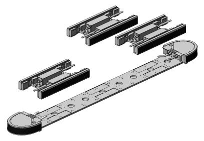
Loosely install four (4) screws into each straight section stand base.
