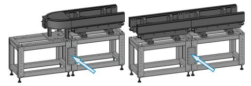
7. Use a 0.5 mm (0.02 in.) shim to verify that a 0.5 mm (0.02 in.) space exists between the aluminum surfaces of section A and section B.
