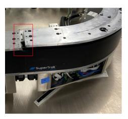
7. Slide the upper v-rail out in the forward direction clear of the motor.
