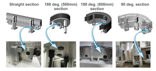
d. As required, remove the black plug in the section before connecting.
