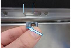
b. Install a screw to secure the locator in position.
