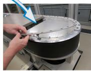
6. Disconnect the RJ11 plug from the encoder assembly connection.
