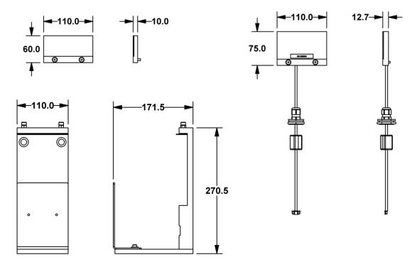
Dimensions for reference only. See SuperTrak Design Package for detailed drawings.
