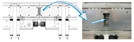
The image below provides a top view of two straight sections that are not aligned.
