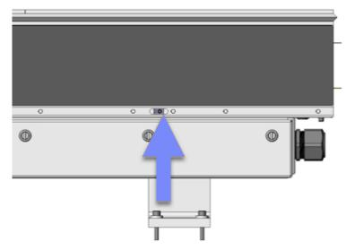
17. Install the wear strips to the straight sections.
