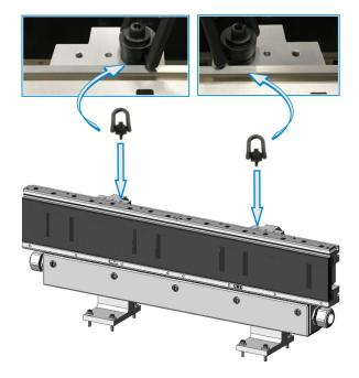
2. Attach each end of one (1) lifting strap to an eye bolt.
