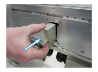
shunt requires iron-to-iron contact with the motor core of each straight section.
