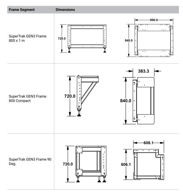
Dimensions for reference only. See SuperTrak Design Package for detailed drawings.
