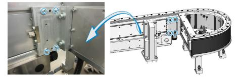
c. Turn the height adjustment screw as required to adjust the upper v-rail height (up or down).
