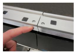
If you feel a ridge, or if the shuttle makes any knocking sounds as it rolls over the upper v-rail joint, continue with the steps in the Adjust the Upper V-Rail ±0.05 mm (±0.002 in.) Straight to Straight or Straight to Curved instructions that follow immediately below.
