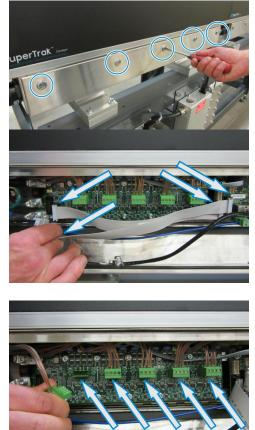
6. Remove the fourteen (14) screws that secure the coil driver board to the bus bar.
