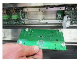
10. If the Gateway board is being returned for repair, remove the hardware (screws, washers, and spacers), and make sure the Gateway board is packaged in an ESD safe bag.
