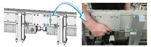
c. Turn the height adjustment screw as required to adjust the upper v-rail height (UP or DOWN).
