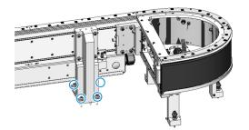
b. Loosen the four (4) wedge screws.
