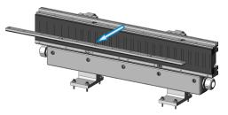
7. Clean the top of the straight section with a soft cloth to remove any debris.
