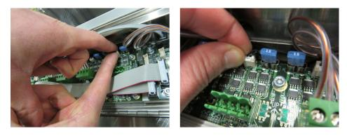
6. Pull the old thermistor wire straight out from the thermistor hole.
