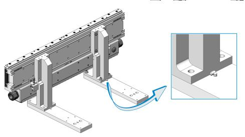
6. Loosely install four (4) screws into each stand base.
