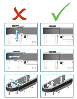
For 180 deg. (500 mm) sections: Remove the top cover form the 180 deg. section, remove the covers from the 180 deg. section stands, and then level the 180 deg. section.
