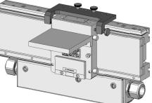
4. Lightly tighten the side thumb screw to lock the shuttle in position against the datum. The side thumb screw has an integrated slip clutch to prevent over-tightening.
