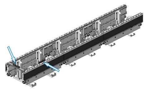
15. Repeat steps 10 to 12 for the remaining sections on the same side of the SuperTrak conveyance platform.
