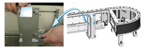
b. Loosen the four (4) wedge screws.
