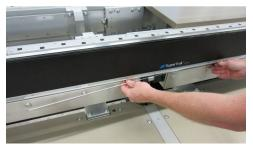
Remove any dirt or debris from the flat wear strip channel.
