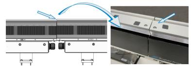
The image below illustrates a possible validation process, where two (2) indicators are mounted to a shuttle to measure the offset between the two (2) upper v-rails.
