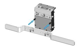
b. Slide the shuttle removal tool to the left, to locate the shaft of the two (2) shoulder screws into the tool slots.
