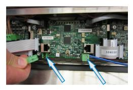
5. As required, unplug one (1) or two (2) motor network connection cables.
