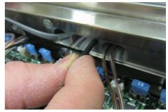
Slide the end of the new thermistor wire into the thermistor hole until you feel resistance. The thermistor tapers. During installation, the thick ridge creates a friction fit against the sides of the thermistor hole.
