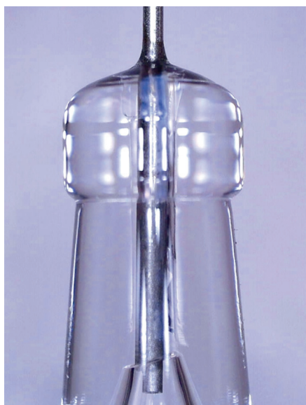
Figure 1: UV-cured adhesive bonding needle to syringe.
