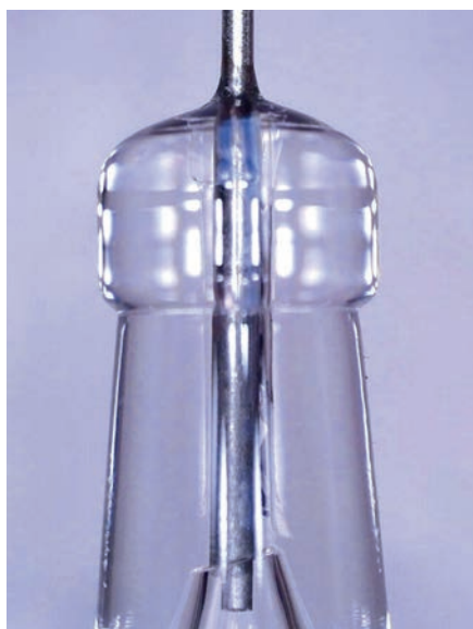
Figure 1: UV-cured adhesive bonding needle to syringe.
