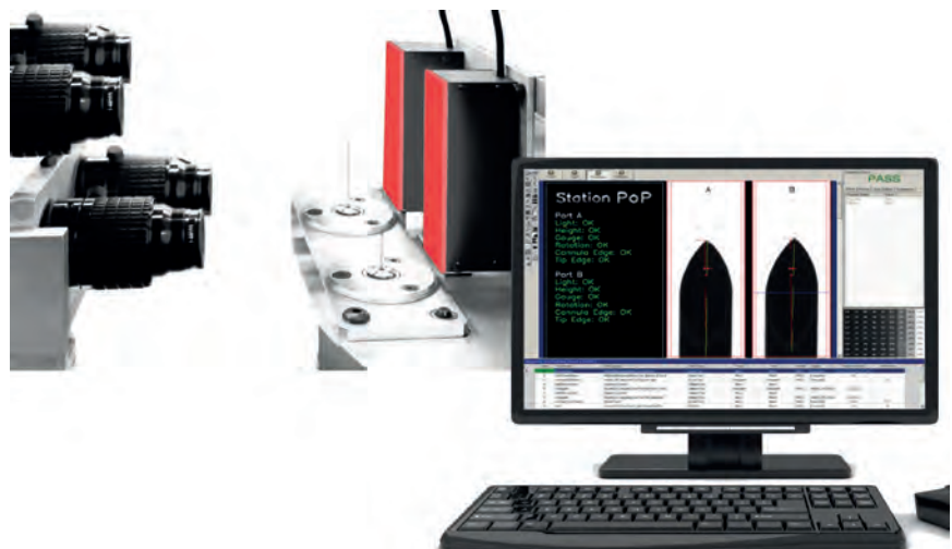
Figure 4: ATS’ vision group demonstrates the ability to identify cannula bevel, defects, orientation, etc.
