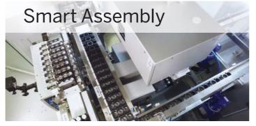
Joining of lids, inserts, and other small assemblies during transfer from tray to assembly areas including test position for correct application etc.
