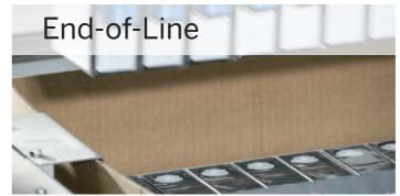
Loading and unloading of cardboard boxes, handling of single boxes with lid application. Optional closing with adhesive strips or stretch banding and many others.
