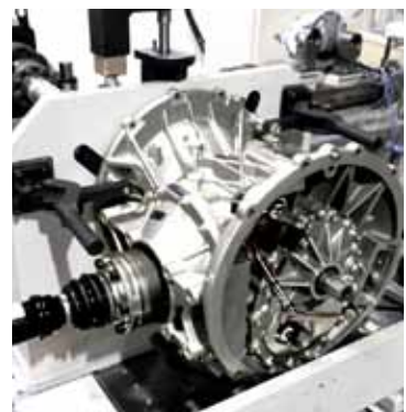
Electric transaxle involving power transfer end of line testing and NVH
